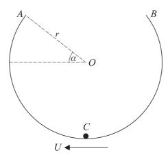
A smooth metal strip with ends A and B is bent into a major arc of a circle with centre O and radius r. The strip is fixed in a vertical plane with AB horizontal and at a height  $r \sin \alpha$  above O, where  $0 < \alpha < \frac{1}{2}\pi$  (see diagram). A particle is projected from the lowest point C with speed U so that it travels along the inside of the strip, reaching A with speed V. The particle then moves under gravity, and arrives at B. Air resistance may be neglected. Show that
