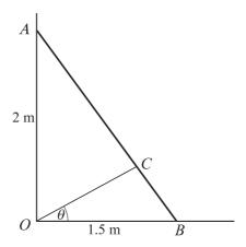
A uniform ladder AB, of weight W N and length 2.5 m, rests against a smooth vertical wall OA with its foot on smooth horizontal ground OB. The ladder is in a vertical plane perpendicular to the wall. It is kept in position with OA = 2 m and OB = 1.5 m by a light rope OC joining O to a point C on the ladder, such that angle  $COB = \theta$ . Show that the tension T N in the rope is given by
